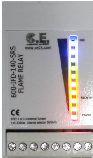
10th led (LIGHT BLUE LED): maximum air ionisation
